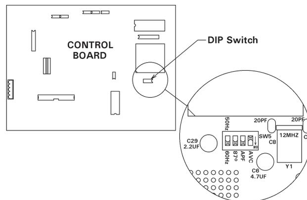
**Figure 2-2.** *EXTENDED FUNCTIONS DIP switch*
