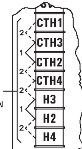
**Figure 9-1.** Voltage Operation jumpers settings
