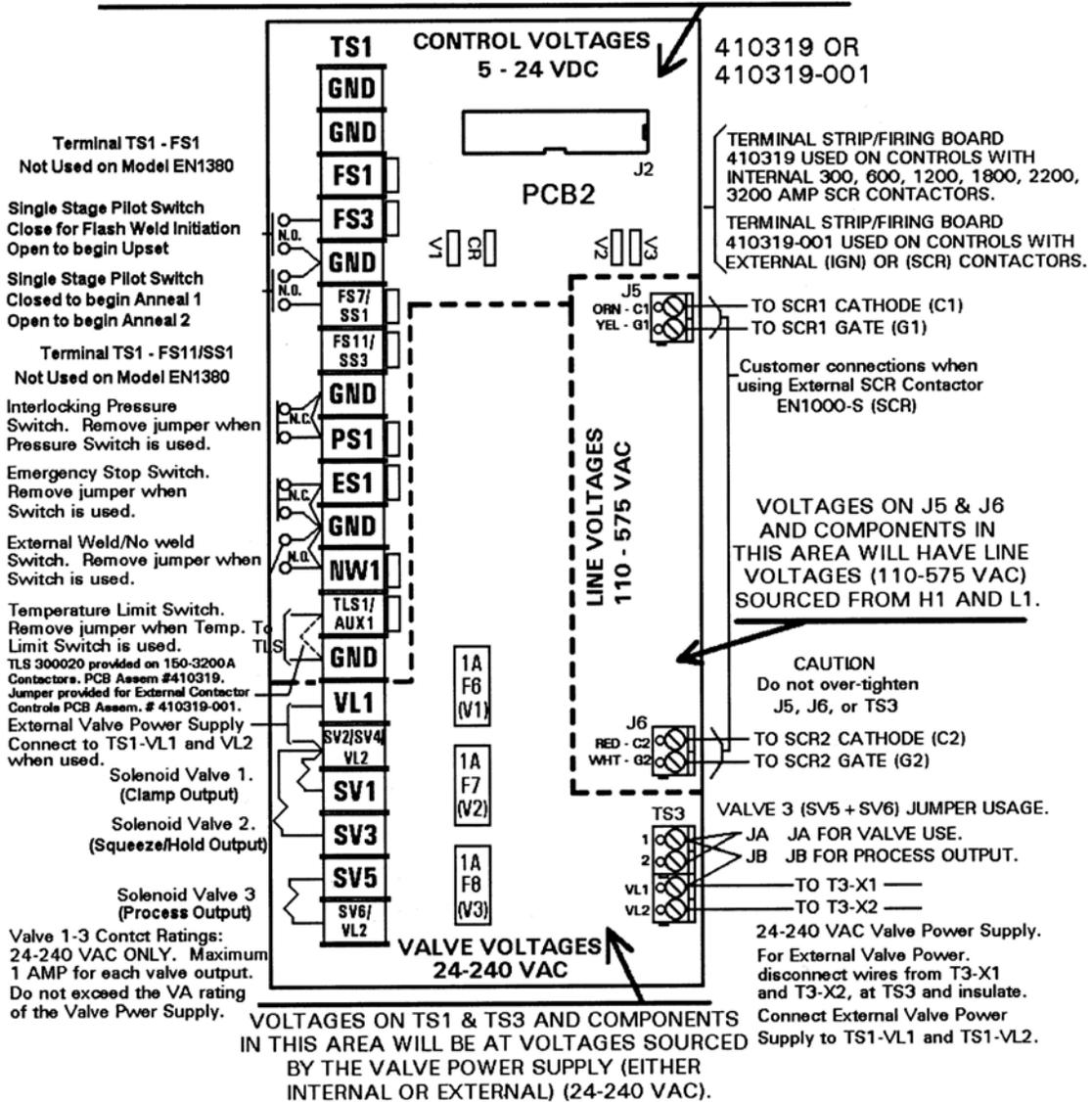
Figure 5-2. Terminal Strip/Firing Board
