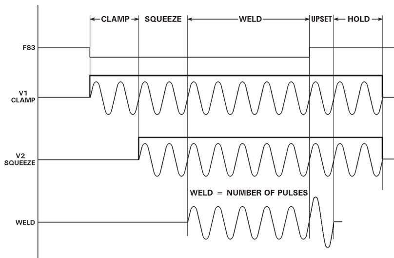
**Figure 3-1. FLASH WELD (BEAT) initiated on FS3 – S.E.=01**
