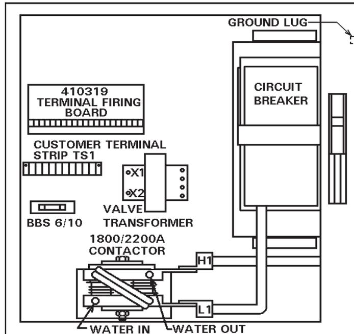
Figure 8-6. “T/D” and “L” Cabinets – 1800/2200A Contactor
