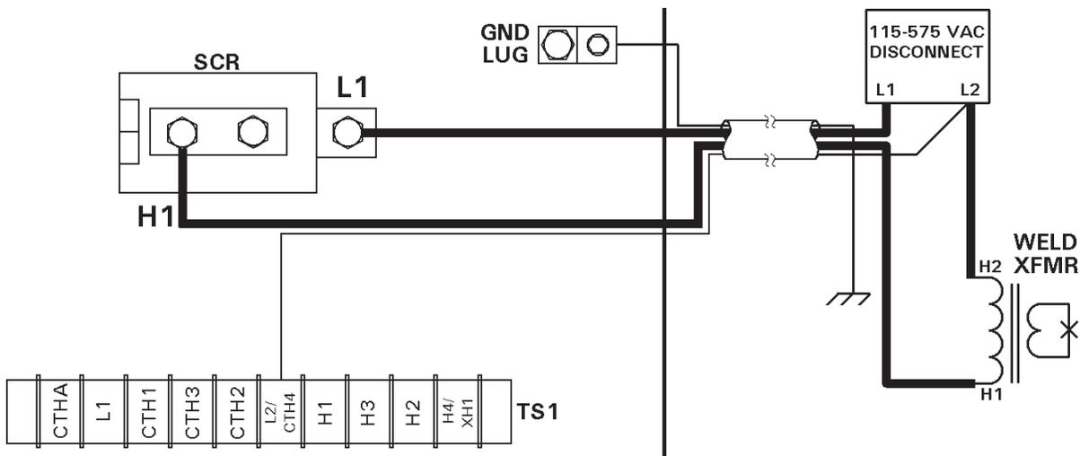
**Figure 5-3.** *Welding contactor connections*
