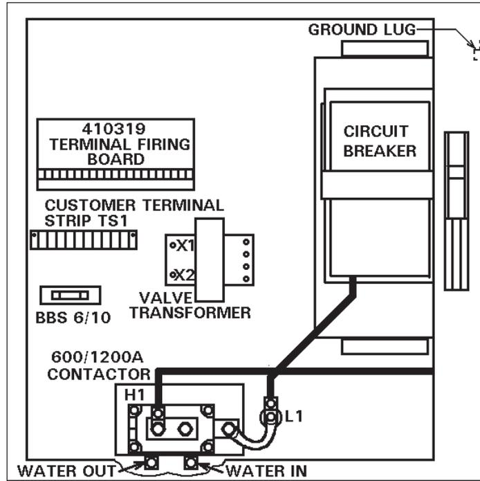
Figure 8-5. “T/D” and “L” Cabinets – 600/1200A Contactor
