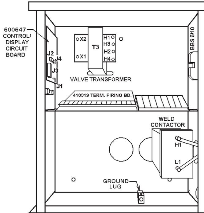
Figure 8-3. "E" Cabinet – 300/600/1200A Contactor
