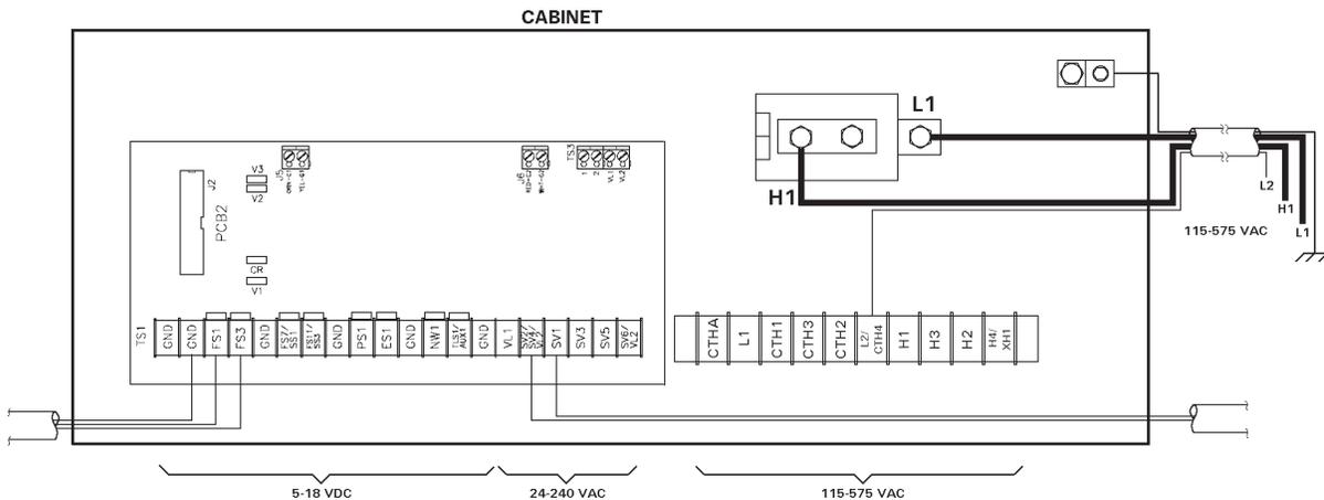
**Figure 4-1.** Recommended wiring and routing
