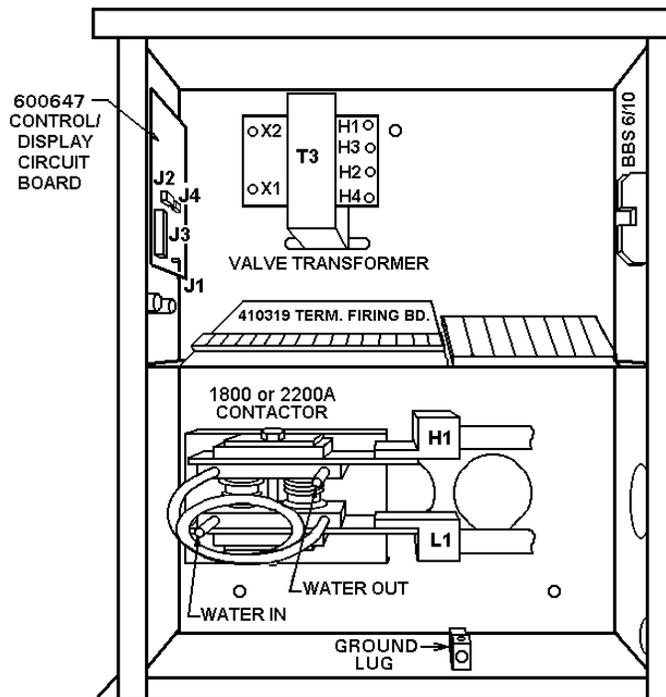
Figure 8-4. "E" Cabinet – 1800/2200A Contactor
