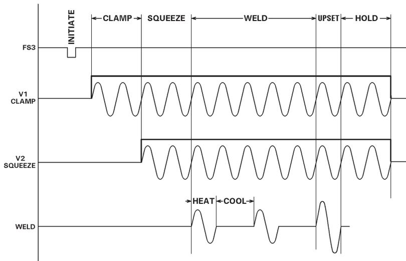
**Figure 3-3. BUTT WELD (NON-BEAT) initiated on FS3 – 5.E.=02**
