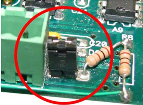
Figure 7-10. Sinking Sensor Jumper detail
