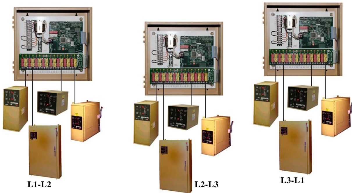
Figure 2-6. Interconnection of Welder Interlocks in a 3-phase system
