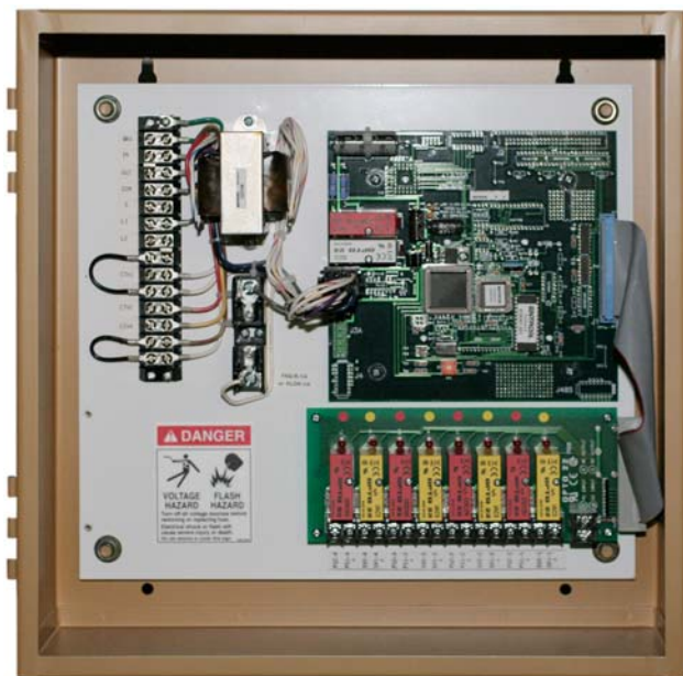
Figure 2-2. Detailed board and harness layout
