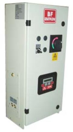
Control cabinet with door-mounted timer, up to 8 programs. Fitted into a sheet steel enclosure with circuit breaker, 24 VDC air valve power supply, appropriate line fusing, safety covers, and an air-or water-cooled SCR power module.
