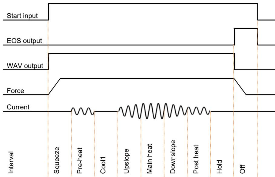
**Upslope** can be used on hard, irregular shaped, oxidized and aluminium materials
