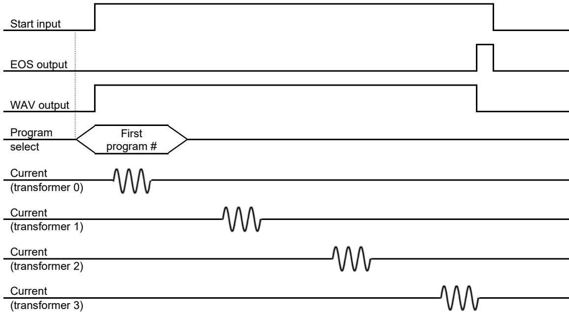
**In multi-gun cascade operation** the program select inputs select the first program in the cascade.
