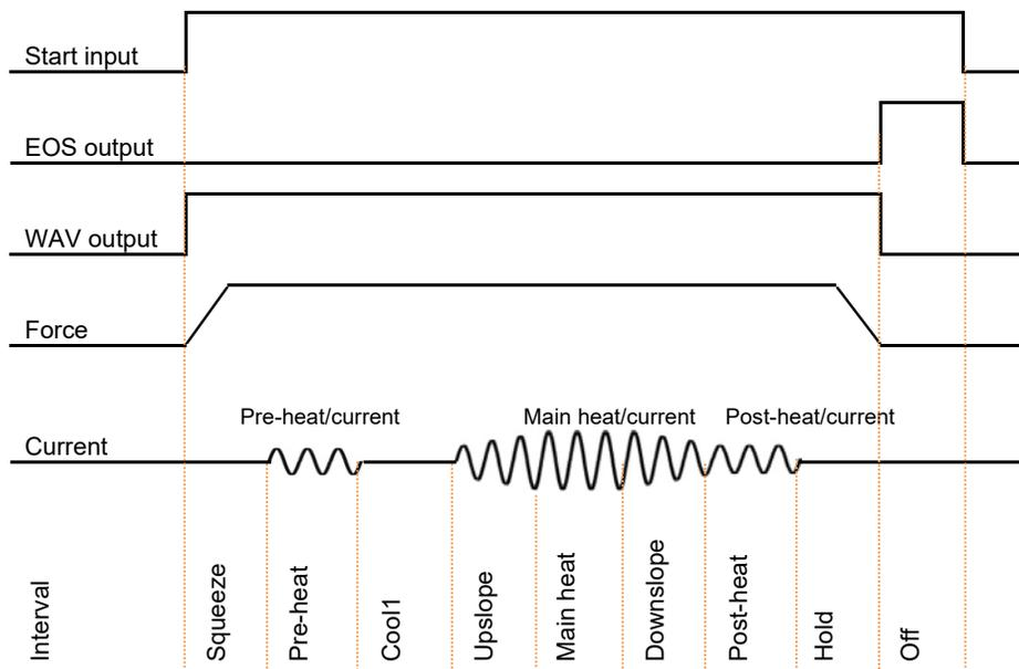
**Pre-heat and Post-heat** can be used on hard or heat resistant metals
