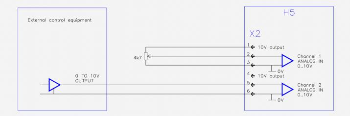
Note that the H5 analog inputs are referenced to 0V (X1 pin 2). If the external equipment requires an isolated connection, then the control signal should be connected to the H5 via a signal isolation amplifier. e.g. BF Entron ISOAMP, part no. 90-90-61
