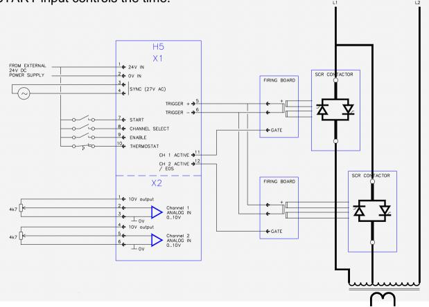
Note that special firing cards having a GATE input are required.
