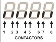
**Figure 5-3.** Contactor indication in DATA display
