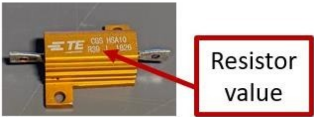
Figure 2 Standard Burden Resistor value R39
