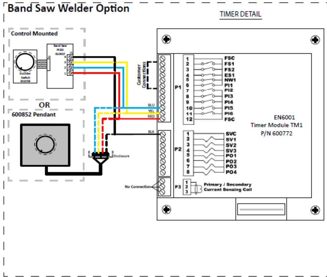
**INPUTS – All inputs are 24VDC from FSC (Footswitch Common) :**
