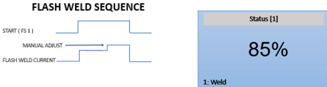
POST-HEAT can be programmed as a timed interval. Post-heat automatically follows Flash Weld when FS1 is released.
