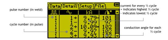
For DC welds, the ½ cycles are replaced with the cumulative weld time in ms. The conduction angle is not applicable to DC welds. The ▲ and ▼keys may be used to
