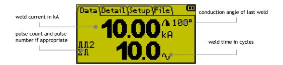
For DC welds, the weld time is shown in ms and cycles. The conduction angle is not applicable to DC welds.
