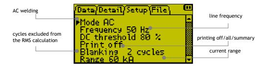
The **Mode** parameter determines the type of welding current to be measured, AC or DC.
