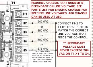
F1-5 on T1 and T2 (optional) may be one of the following 1-1/4 A fuses (FNQ, KLDR, ATQR, TPK - 1 1/4 A. These 5 fuses protect control circuitry.
