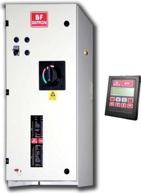
Control cabinet with door-mounted timer, up to 64 programs, constant current control and monitoring. Fitted into a sheet steel enclosure with circuit breaker, 24 VDC air valve power supply, appropriate line fusing, safety covers, and a direct water-cooled or air-cooled SCR power module. Optional hand-held pendant.
