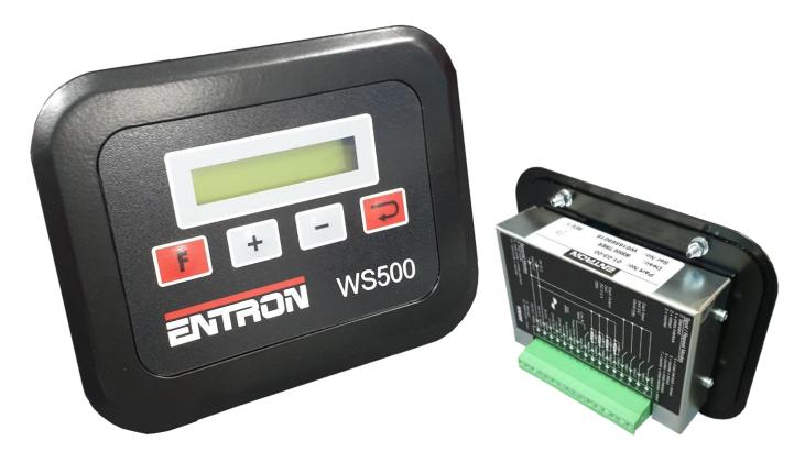
The WS500 is a high accuracy resistance welding timer intended for use in conjunction with almost any type of resistance welding machines. The user programming is very simple using a built in tactile keypad in conjunction with an back lit LCD. The timing is controlled and set in terms of one cycle increments based on the supply frequency (50 or 60 Hz). The WS500 provides eight programs and a versatile range of functionaloty as shown overleaf.
