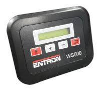
The WS500 is a high accuracy resistance welding timer intended for use in conjunction with almost any type of resistance welding machines. The user programming is very simple using a built-in tactile keypad in conjunction with an back lit LCD. The timing is controlled and set in terms of one cycle increments based on the supply frequency (50 or 60 Hz). The WS500ms provides eight programs and a versatile range of functionality as shown overleaf.
