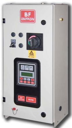
Control cabinet with door-mounted timer. Fitted into a sheet steel enclosure with circuit breaker, 24 VDC air valve power supply, appropriate line fusing, safety covers, and a direct water-cooled or air-cooled SCR power module and Primary CT for current regulation.
