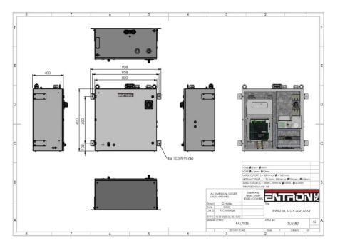
Complete engineered welding control in self-contained easy to install cabinet, including safety screens, circuit breaker with door interlocking, optional isolation contactor, power supplies and earth leakage protection.
