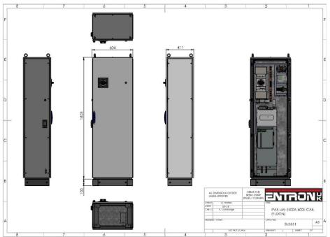
Complete engineered welding control in self-contained easy to install cabinet, including safety screens, circuit breaker with door interlocking, optional isolation contactor, power supplies and earth leakage protection.
