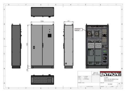
Complete engineered welding control in self-contained easy to install cabinet, safety screens, circuit breaker with door interlocking, optional isolation contactor, power supplies and earth leakage protection.
