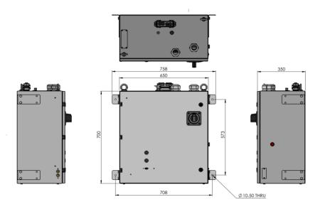
Complete engineered welding controls in self-contained easy to install cabinet, including safety screens, circuit breaker with door interlocking, power supplies, optional isolation contactor and earth leakage protection.
