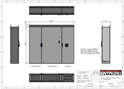
Complete engineered welding control in self-contained easy to install cabinet, including safety screens, circuit breaker with door interlocking, power supplies and earth leakage protection.
