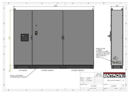
Complete engineered welding control in self-contained easy to install cabinet, including safety screens, circuit breaker with door interlocking, power supplies and earth leakage protection.
