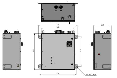
Complete engineered welding control in self-contained easy to install cabinet, including circuit breaker with door interlocking, safety screens, optional isolation contactor, power supplies and earth leakage protection.
